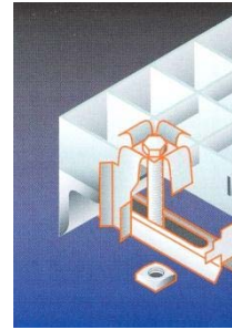
Standard fastener • Locking clip upper part • Clamp lower part • Hexagon screw M8 • Square nut
