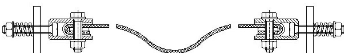
using the turnscrew to make the mesh tight
