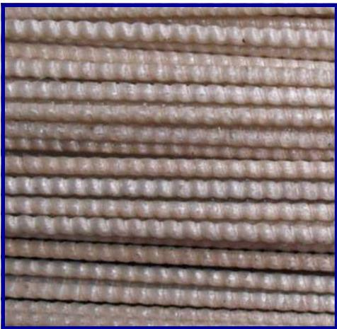
**PowerBar** is manufactured by pultrusion process with in-line winding and sand blasting on the surface to provide bond adhesion to concrete.
